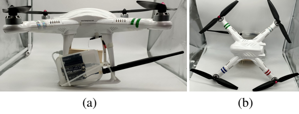
Figure 2. UAV equipped with LoRa receiver. (a) Side view and (b) top view.
